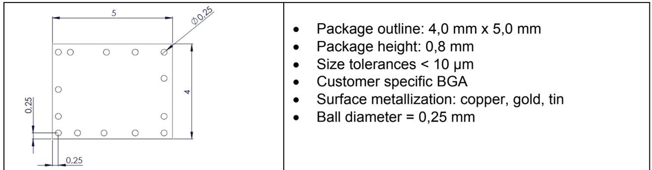
Figure 2: Package dimensions and interface specification
