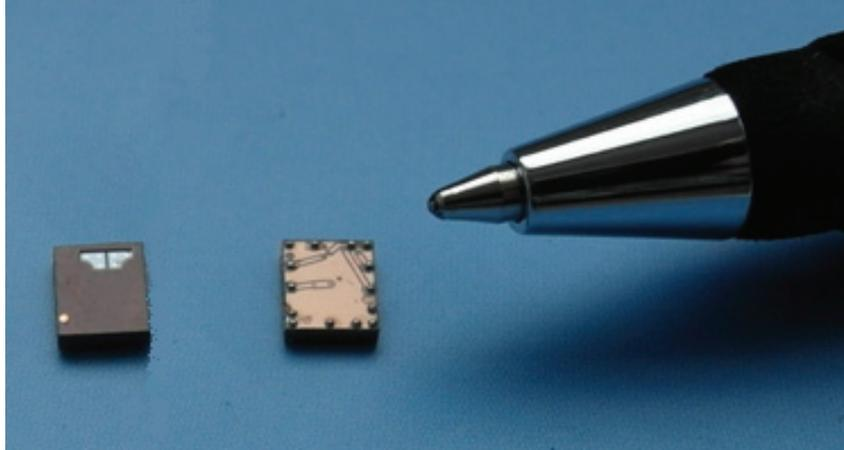
Figure 3: Sensor package solution: Top side (left) and bottom side (right)
